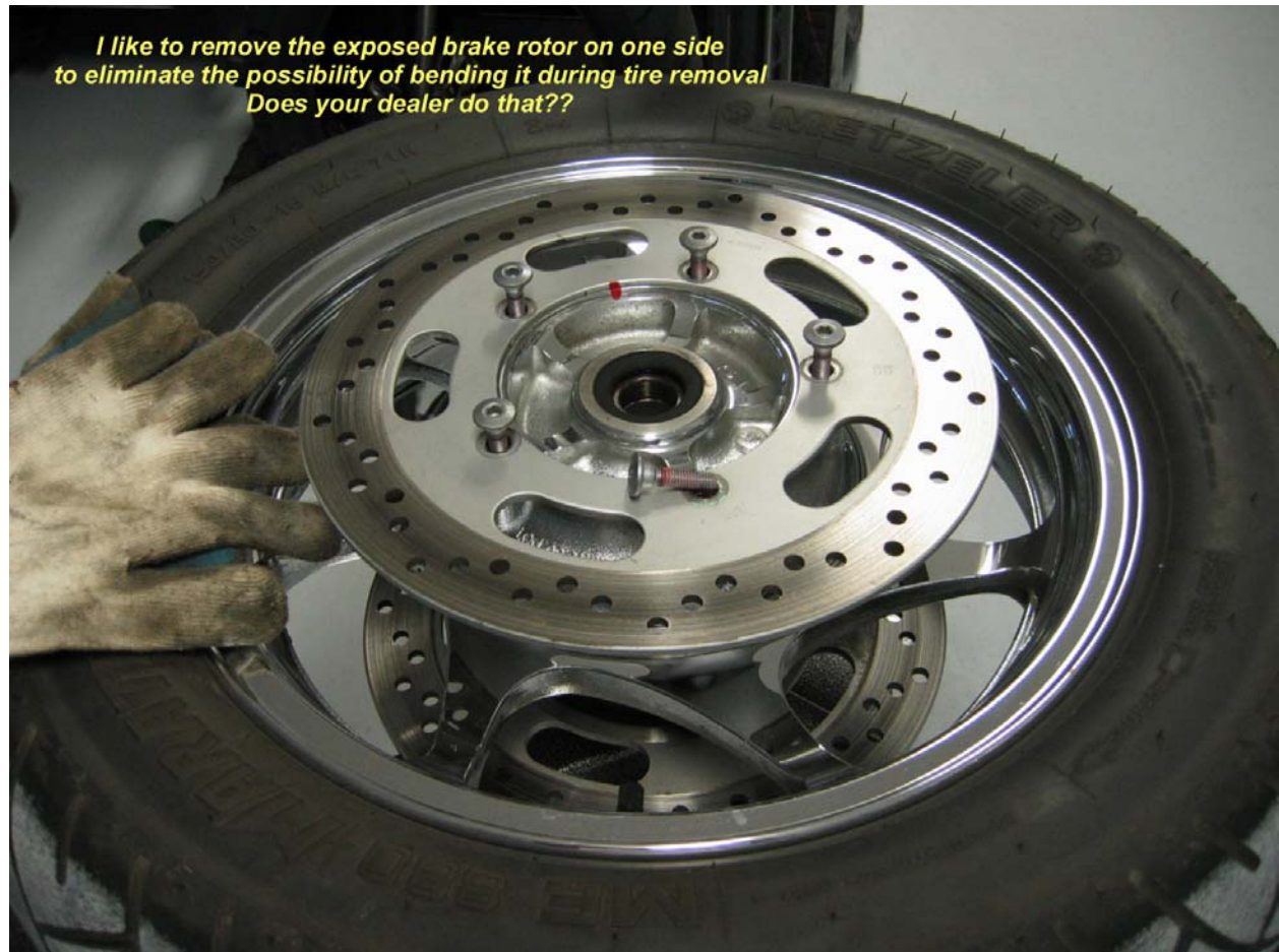
Note the red alignment mark I added to be sure the rotor goes back on in the same orientation.
