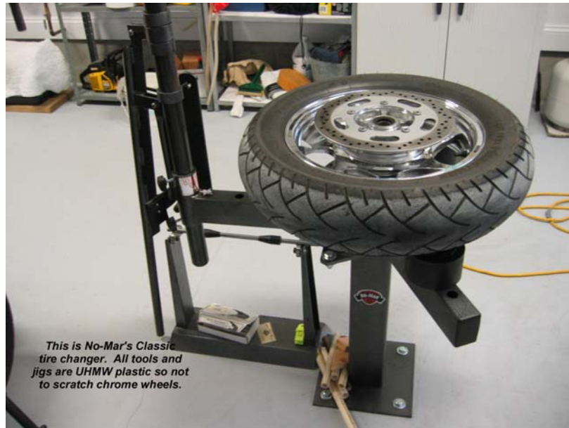
I like to remove the exposed brake rotor on one side to eliminate the possibility of bending it during tire removal. Does your dealer do that??
