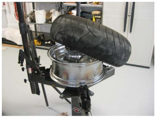
Note the rim clamps on the tire changer – these are optional equipment on the No-Mar changer and definitely worth the cost as they don't tend to slip and do not get in the way of the tire sidewall during installation.
