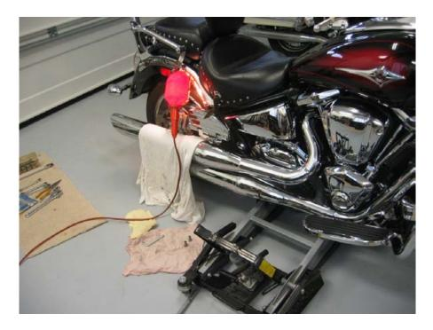
Up on the lift she goes – I put a rubber band on the front brake lever just as added precaution that the bike won't tend to roll forward when the weight of the rear tire is not there to balance the load.
