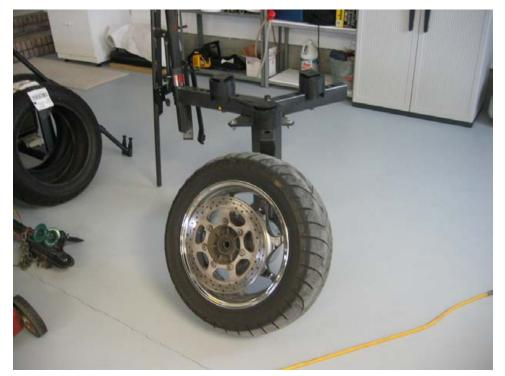
Here we are ready to remove the valve core and let the air out, then mount the tire on the No-Mar tire changer. Do not lay the tire down on the brake disc – this could warp the disc and cost you big \$\$ to replace.
