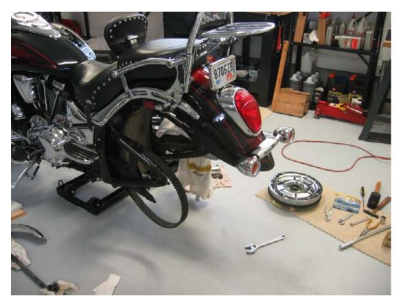
Now raising the bike up allows the tire to be rolled out. I've removed the drive pulley; it takes a little coaxing to pull it off the wheel due to the tightness of the rubber shock absorbers. The first time the drive pulley was removed was a chore. I apply Never-Seize to the rubber and to the pulley. The pulley slips off much easier now.
