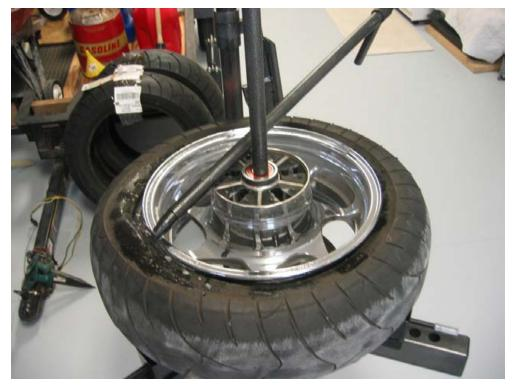
Got the bead broken and the removal tool ready to remove the tire - using some slick spray lubricant makes the removal easier. This is the easier part of manual tire changing.
