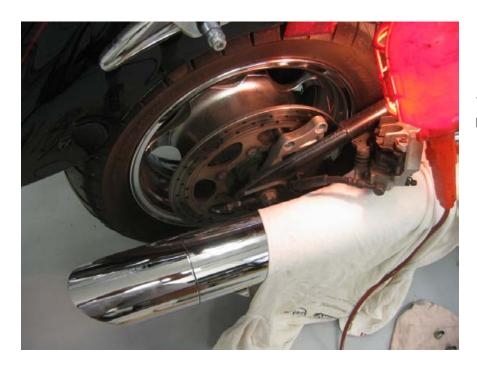
Caution: do not touch the rear brake lever until the calipers are re-installed or the brake pistons could be pushed out of the caliper!!
