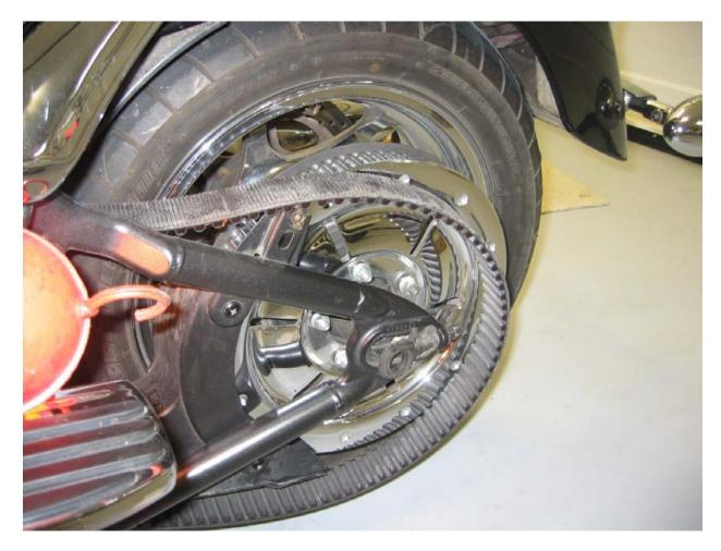
I removed the cotter pin, axle castle nut, and the axle. It's easier for me to use the lift to just unweight the tire assembly by having it just touch the floor – that makes pulling the axle very easy. Now after loosening the belt adjusters, the tire has been rolled forward and the belt easily comes off. Belt looks good for 47,000+ miles (no cracks, breaks, missing teeth, etc. – just a little dry; I'll spray it with silicone at reassembly to keep it quiet for awhile).
